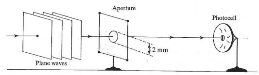
In this situation, the radius of the *m*-th Fresnel zone can be approximated as:  $R_m = \sqrt{m \ r_0 \ \lambda}$ , with  $r_0$  the distance of the photocell to the aperture.
